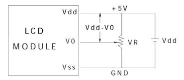
Vdd-V0: LCD Driving Voltage
