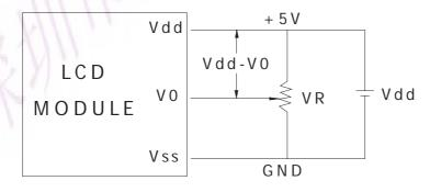
$Vdd\hbox{-}V0\colon LCD\ Driving\ Voltage$
