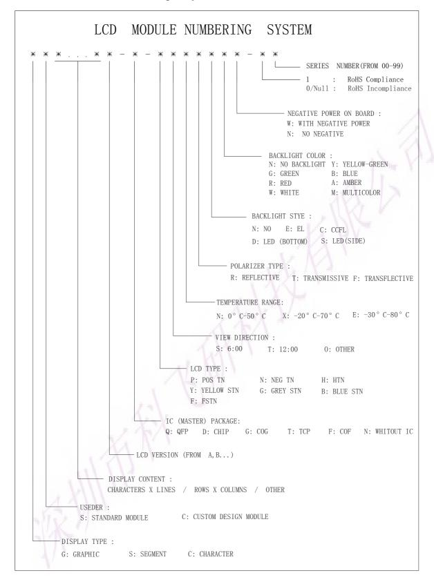
1. LCD Module Numbering System
